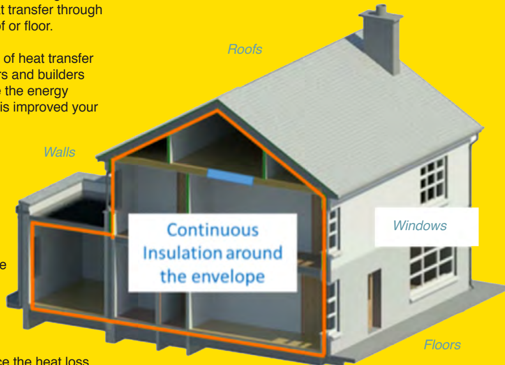
Continuous insulation shown by the orange line eliminates heat loss through the envelope
